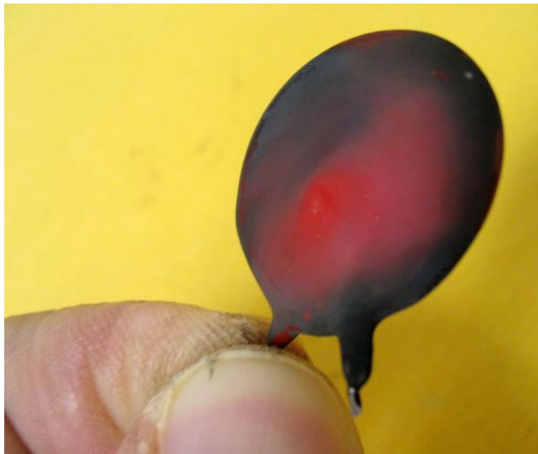
Figure 6-4 Crispy Factor of CF0, Indicating an Intact MOV Even If Covered With Soot From Other MOVs
