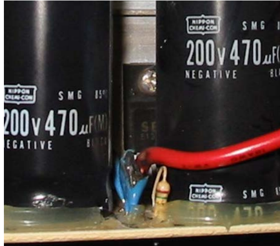
Figure 6-7 MOV Failure Inside the Computer Power Supply of PC4
