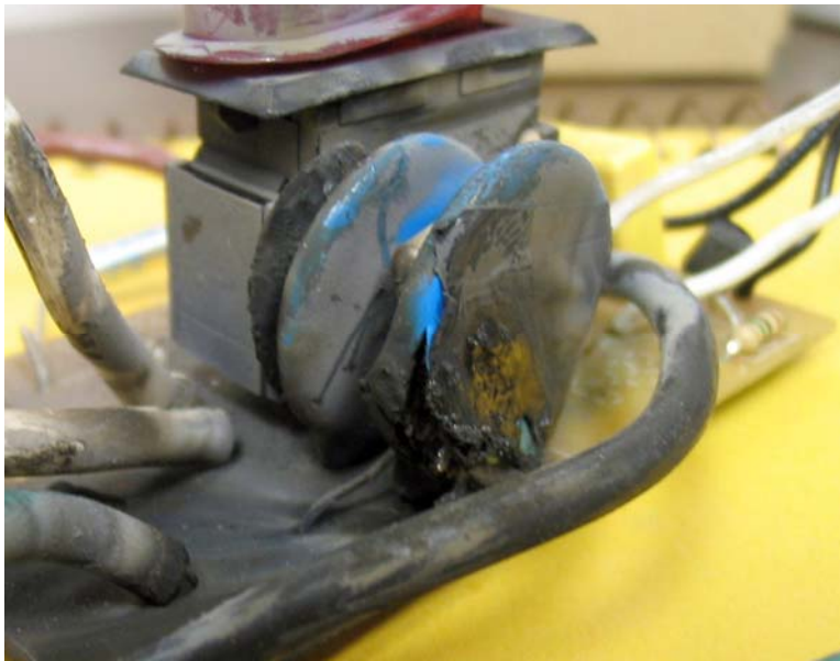
Figure 6-2 Crispy Factor of CF2, Indicating a Flaky Surface and Some Loss of Physical Structure
